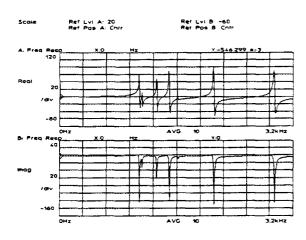
Now the analyzer displays real and imaginary instead of magnitude and phase. Note that the imaginary components all point in the same direction. This is characteristic of a driving point measurement.
