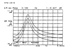
This turns on the limit test evaluation. When test evaluation is on, you can see a message at the bottom of the display that indicates if the device-under-test has passed or failed the limit test.
