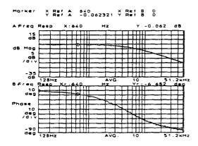
Marker coupling means that markers for both the upper and lower trace move at the same time when you turn the knob.
