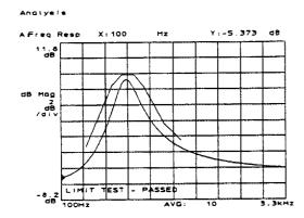
This turns on the limit test evaluation. When test evaluation is on, you can see a message at the bottom of the display that indicates if the device-under-test has passed or failed the limit test.
