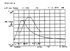
In the example here, we changed the center frequency of the test filter from 1 kHz to 500 Hz.
