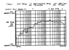
In the example here, we measured a typical desktop impact printer, without a noise shroud (this is track 10 of the demonstration disc). As you can see, the total A-weighted SPL is about 60 dB.
