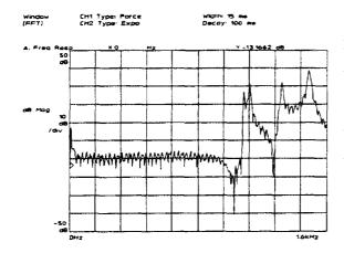
This trace shows the frequency response of multiple impact, such as when the hammer bounces during impact. Notice that a multiple impact produces a ripple on the frequency response.
