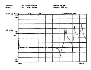
This trace shows the frequency response of a single, good hammer tap.
