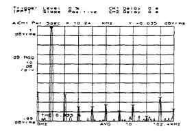
This begins a new measurement. Notice how the noise floor lowers and how much easier it is to view harmonics of the sine signal.
