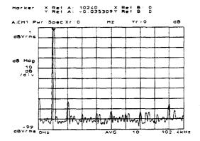
This turns on the relative marker and zeroes it at the marker current marker position. Both X and Y marker readouts are now set to zero—this point now becomes the reference.
