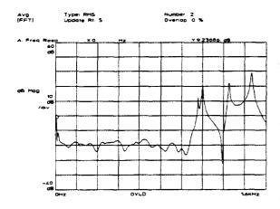
This trace shows the frequency response with channel 1 overloaded. Notice that the overload causes distortion in the frequency response.
