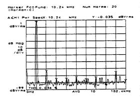
This turns on the harmonic distortion marker and sets the fundamental frequency to equal the current marker position—in this case, 10.24 kHz.
