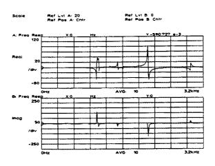
In this example, the resonant frequencies in the frequency response are the same as the previous example, but the relative amplitudes at each resonance are different. Notice that the imaginary components do not all point in the same direction.
